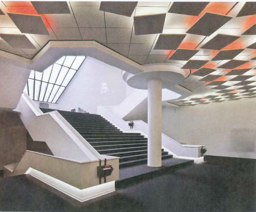
Below: The felt-clad acoustic tiles conceal lights that not only change color and intensity but act as way-finding devices and cues for audience members to take their seats.
